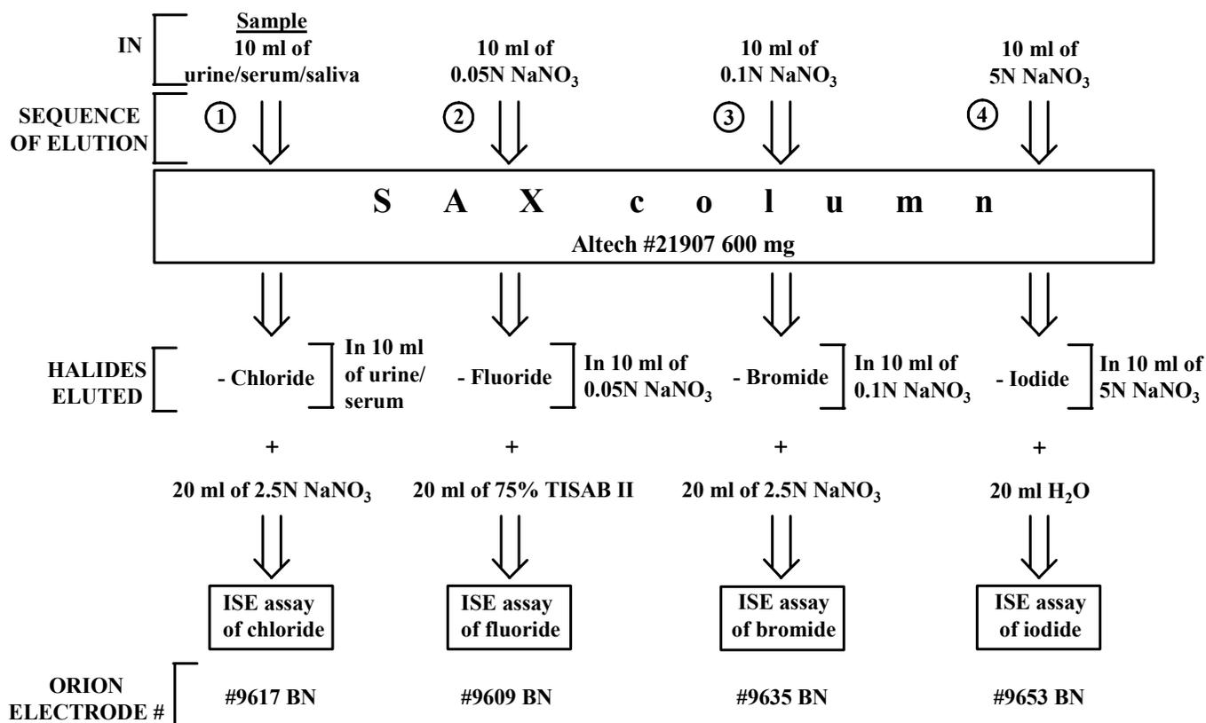
Chloride, fluoride, bromide, and iodide measured by prior chromatography on the anion-exchange resin cartridge SAX 600 mg fitted with 10-milliliter plastic syringes in a positive displacement manifold.<sup>12</sup>
